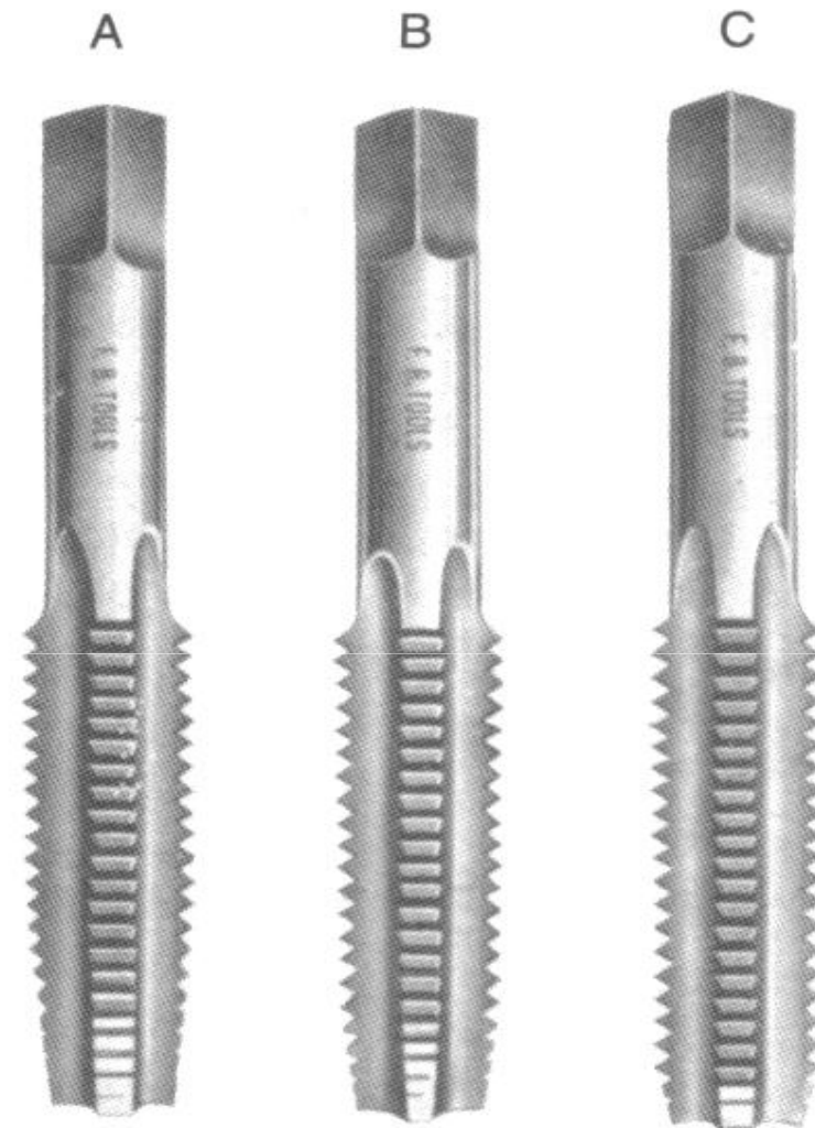
A set of hand taps: (A) Taper; (B) plug; (C) bottoming.
